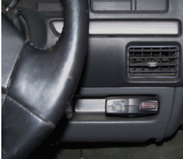
FIGURE 1-14 This is a typical add-on trailer brake controller.
