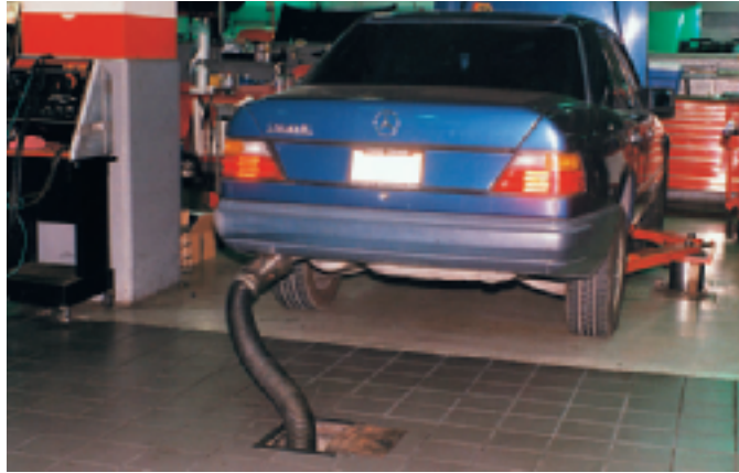
FIGURE 1-4 When running an engine in a shop, always connect the exhaust to the ventilation system.
