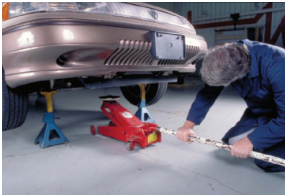
FIGURE 1-2 Support a vehicle on safety stands such as these and move the jack out of the way.
