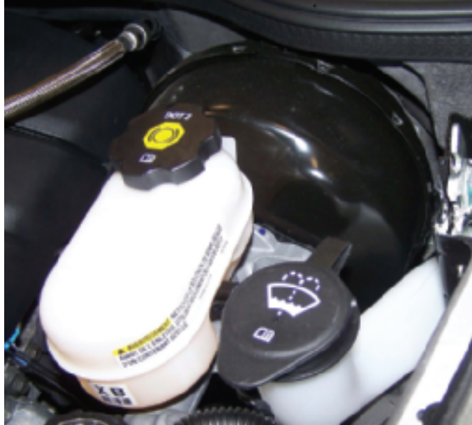
FIGURE 1-13 The power brake booster increases the brake pedal force applied to the master cylinder.
